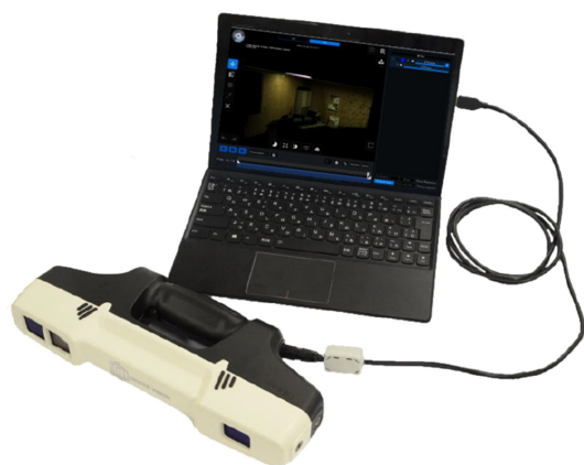
Fig. 1. A handheld three-dimensional laser measurement device connected to the laptop by USB cable.
