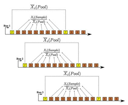
**Fig. 1.** Normalization by reference pool measurements. In a GC-MS sequence plan, every 8th position a reference pool sample is measured. For pool normalization, the average of the 2 nearest pools is calculated for each metabolite i ( $\overline{X_i}$ ). Then, for each sample the metabolite intensity of each metabolite i is divided by the corresponding average  $\overline{X_i}$  of the pools:  $\frac{X_i(Sample)}{\overline{X_i}(Pool)}$ .
