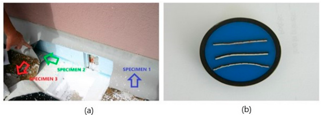
Figure 2. Demonstration of the PVC-P membrane sampling at the facility (a); the Specimen produced for analysis on the stereo optical microscope (b).
