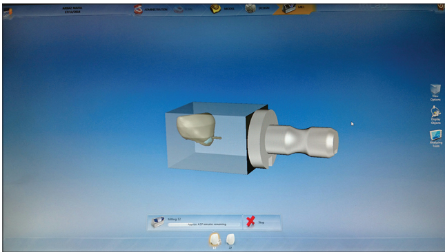
Figure 4: The location of the sprue and position of the crown was adjusted in a polychromatic block
