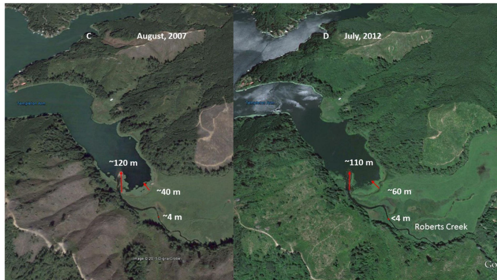
Figure 9. US Geological Survey color aerial images of Tenmile Lake, Templeton Arm, and Roberts Creek. (C) : The August 2007, aerial image shows the Roberts Creek channel is incised, and the delta is expanding. (D) : The July 2012, aerial image shows the Roberts Creek channel is unchanged, and the delta has been reduced by approximately 10 m from the August 2007 image. The August 2007 image also shows increased clear cuts on the slopes in three areas south of (below) the lake. Source: Images obtained from Google Earth. Note : Red arrows show the extent of delta growth.
