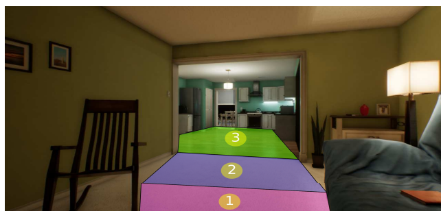
Figure 23. Environment division using navigation meshes for rooms 1 and 2.
