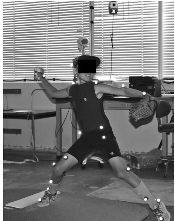
Figure 1. Participant pitching off the portable pitching mound during the simulated game. Shown is 1 of 8 motion analysis cameras (behind the participant at the top of the photo) as well as the retroreflective markers for recording kinematics.
