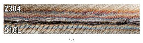
Figure 2. View of the welded joint: (a) face side and (b) root side.
