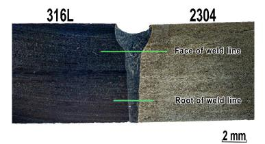
**Figure 5.** Cross-section of the 316L–2304 stainless steel welded joint. The arrangement of microhardness measurement points on the specimen is marked by lines.
