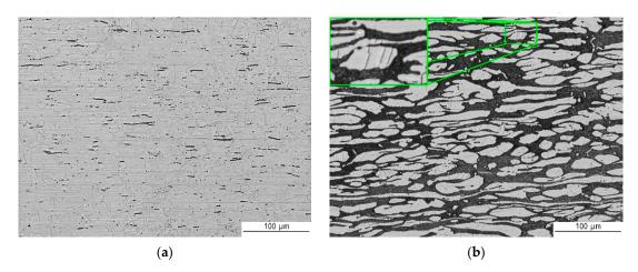
**Figure 6.** Metallographic structure (light microscope (LM)) of: (a) 316L austenitic stainless steel and (b) 2304 duplex stainless steel.
