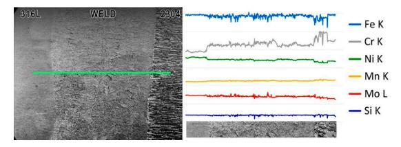
**Figure 9.** Results of EDS linear analysis through the welded joint from 316L austenitic stainless steel (beginning of the line) to 2304 duplex stainless steel (end of the line). The analysis was carried out along the line indicated in the SEM image on the left.
