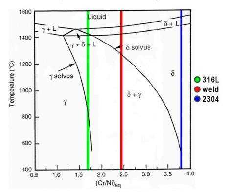
Figure 12. Fe-Ni-Cr pseudo-binary phase diagram.
