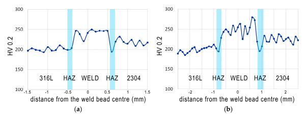
**Figure 10.** Microhardness (HV0.2) distribution across the welded joint: (a) 2 mm below the weld face and (b) 2 mm above the weld root.
