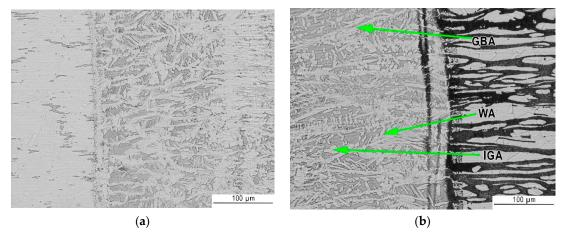
**Figure 7.** Metallographic structure (LM) of: (a) 316L austenitic stainless steel→HAZ→WM and (b) WM→HAZ→2304 duplex stainless steel.
