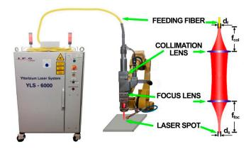
Figure 1. Experimental set-up for fiber laser welding [56].
