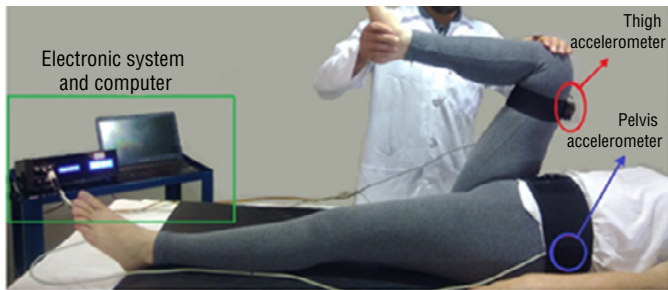
Figure 4. Positioning of pelvic accelerometers (pelvic retroversion estimator) and thigh accelerometer (hip flexion estimator).
