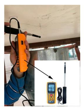
Figure 6. Digital velocity measurement.
