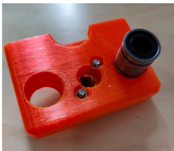
Fig. 4. Fitting the LM8SUU bearings into the Perry Plunger .
