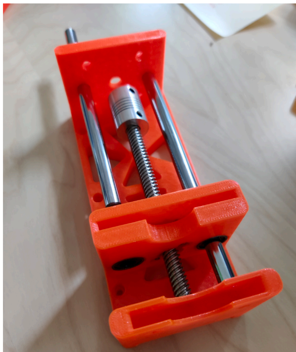
Fig. 7. Installing the Perry Plunger on the smooth rods. Make sure that the smooth rods do not protrude from the top of the Perry Body , as this will cause the motor mounting to be difficult.
