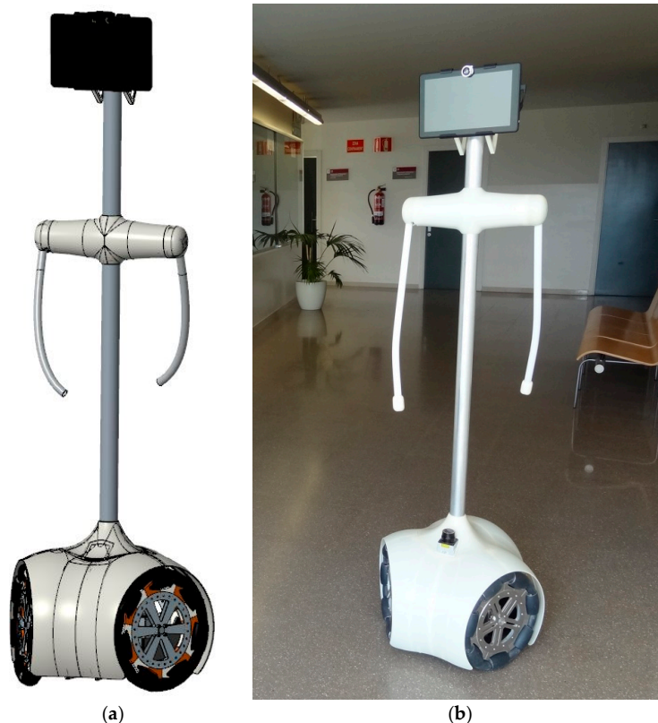
Figure 2. Assistant Personal Robot (APR): (a) CAD design; (b) prototype implementation.
