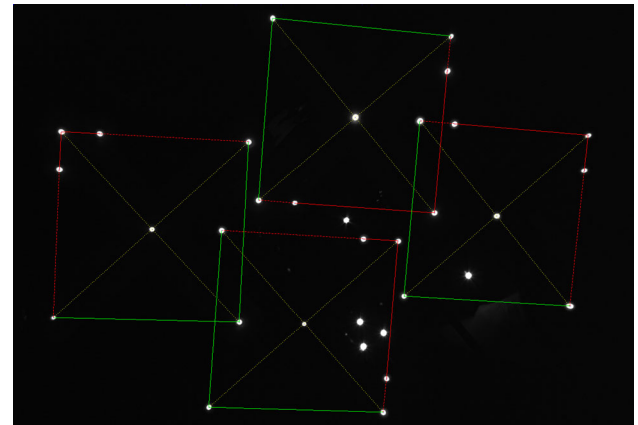
Fig. 9 Marker assignment result for four overlapping trackers with five extra light sources
