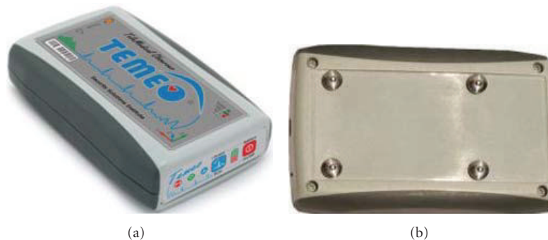
FIGURE 3: TEMEO handheld device: top and bottom view. Four pin electrodes are well seen.
