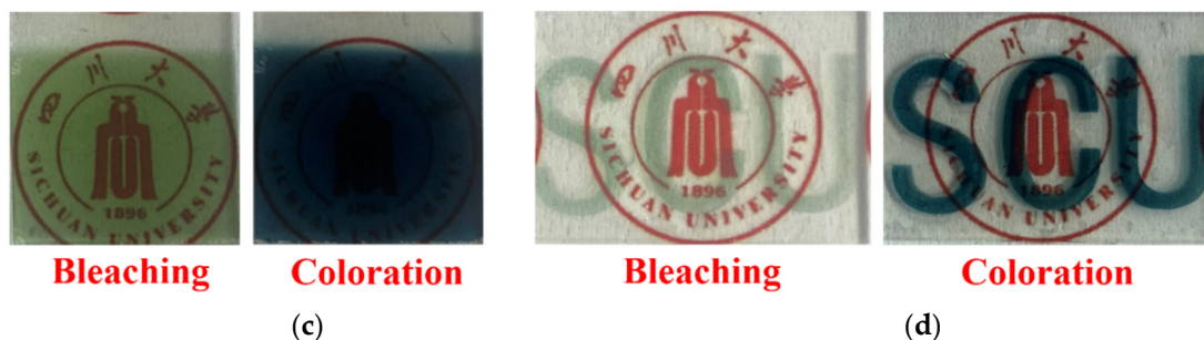
Figure 7. (a,b) Cycling stability testing of PANI and PANI/MXene films for 500 cycles at 700 nm; (c) photograph of PANI/MXene nanocomposite film at -0.4 V (bleaching state) and +0.8 V (coloration state); (d) photograph of the patterning electrochromic film based on PANI/MXene.
