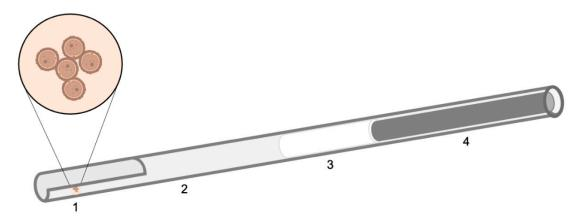
**Figure 1.** Schematic representation of the custom-made minimal volume (<1  $\mu$ L) cryo-device. 1: Droplet of vitrification medium with 4 to 6 oocytes. 2: 0.25 mL straw with a cut in one end to allow loading of the oocytes in a minimal volume (<1  $\mu$ L). E: Cotton of the straw pushed to the middle by the wire. 4: Metal wire, obtained from a paper clip, was inserted to prevent floating in LN2.
