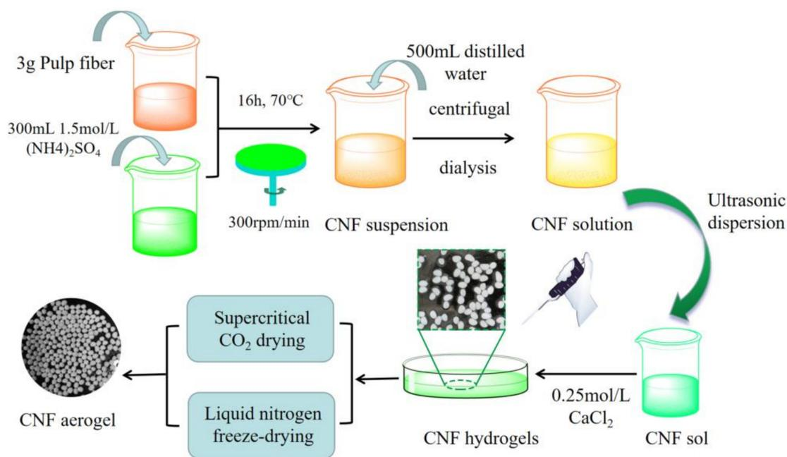
**Figure 1.** Schematic illustration of the preparation processes for cellulose nanofiber (CNF) aerogel via two drying methods.
