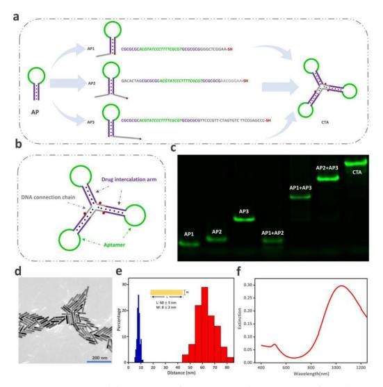
**Figure 1.** Construction and characterization of GNR@CTA. (**a**) Schematic diagram of CTA, (**b**) Functional area division of CTA, (**c**) Gel Electrophoresis Characterization of CTA, (**d**) TEM characterization of GNR, (**e**) Length and width distribution of GNR, and (**f**) UV-visible-NIR spectrum of GNR.
