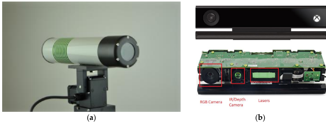
Figure 1. (a) Middleton Spectral Vision MSV 101 Hyperspectral Camera. (b) Kinect V2 depth sensors.
