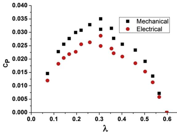
**Fig. 4.** Comparison of coefficient of power ( $C_p$ ) at wind velocity  $V = 7$  m/s.
