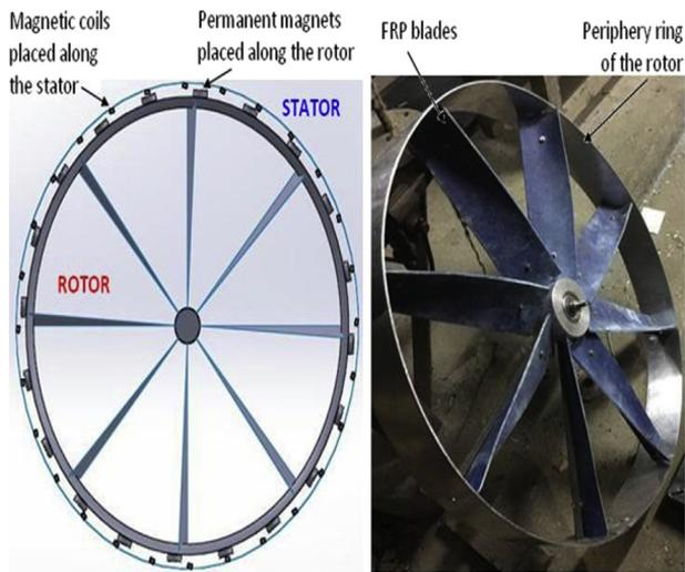
(b) Model of the HAWT with permanent magnets at rotor and magnetic coils at the stator
