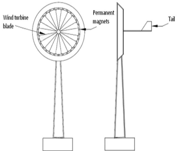
(a) Schematic arrangement of a horizontal axis wind turbine with blade tip power system
