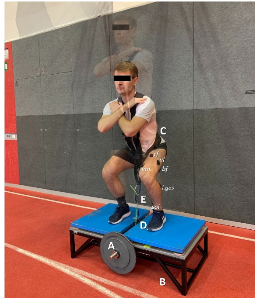
Figure 1. The inertia of a spinning flywheel (FW) (A) produced resistance during squat performance. Subjects stood on a platform (B) (size 1.1 \times 0.6 m), with the pulling rope (with a diameter of 0.006 m) wrapped around the rotating shaft, 0.03 m in diameter. The resistance from the FW device was transmitted to the body by means of a harness (C). The wire of a draw-wire sensor was placed directly above the axis center so to avoid distorting its position due to diagonal vertical displacement (D). The distal draw-wire attachment was in the same location as the harness pulling the rope attachment (which was between the legs) (E).
