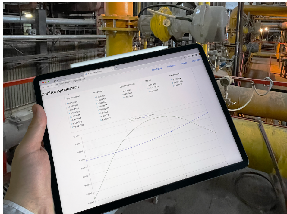
Figure 4. The User Interface of the developed MPC application as used on the factory floor.
