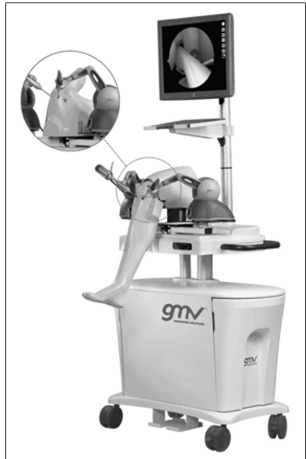
Figure 1. Virtual reality arthroscopy trainer, GMV/insightArthroVR, by courtesy of GMV, Madrid, Spain.
