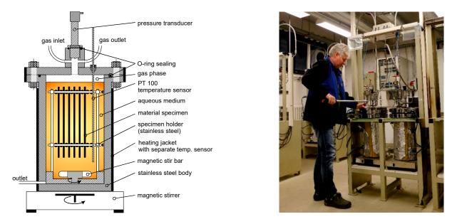
**Figure 1.** Schematic view of autoclave test equipment (**left**), closing the cover plate of the autoclaves (test rig with two autoclaves).
