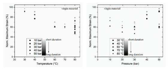
**Figure 4.** Retained elongation  $R_{\varepsilon}$  measured after exposure in autoclaves as a function of temperature (**left**) and pressure (**right**). The duration of exposure is visualized by the gray scale of the symbols. Note that at 80 °C experiments at three different pressures (10, 20, and 30 bar, different symbols) were performed.
