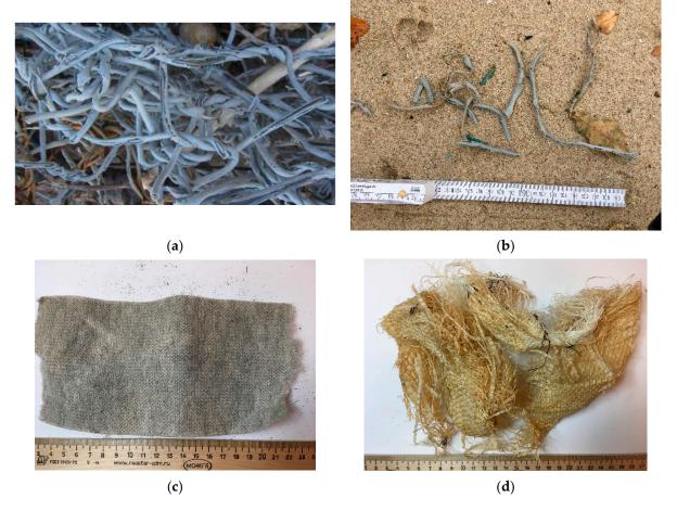
**Figure 3.** Photographs of samples collected during the field study: (a) + (b): aged plastic coating of wires in gabions' (c) debris from geocell; (d): debris from big bag.
