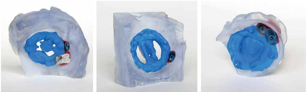
**Figure 3.** Printed PVL models with tested occluders
