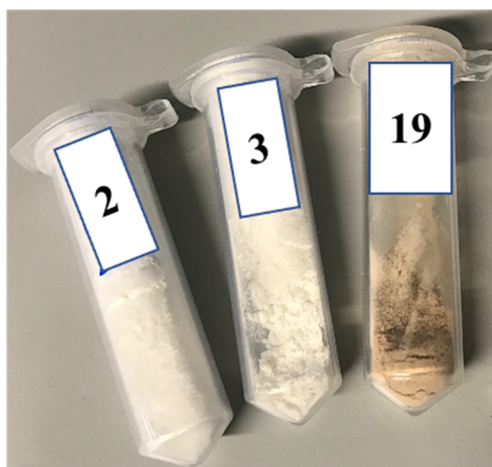
Figure 3. Physical appearance of samples extruded at 100 °C (sample 2), 150 °C (samples 3), and 200 °C (sample 19).
