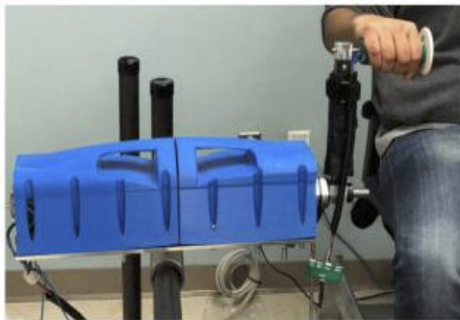
Fig. 1. The Haptic TheraDrive, a one degree-of-freedom rehabilitation robot system used in this study. Image used with permission from [38].
