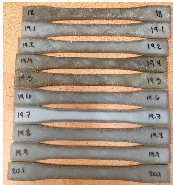
Figure 11. Tensile bars 3D printed with rPET water bottle flake on the adapted Gigabot X and Crammer shown in Figure 2.
