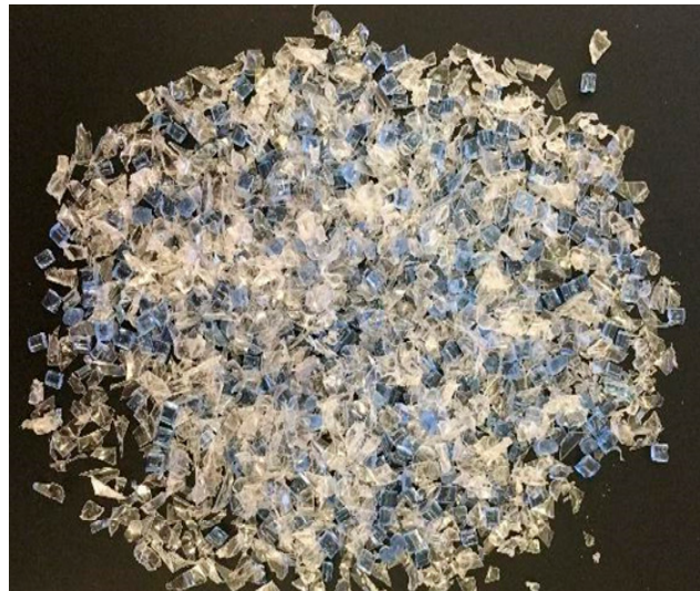
Figure 1. A 50:50 mix of Ultrafuse (blue pellets) and shredded water bottle (clear) to show relative, size, shape, and texture.
