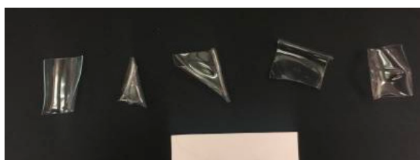
Figure 7. Water bottle squares after 1 h at 100 °C (scale shown with 50.8 mm white bar).
