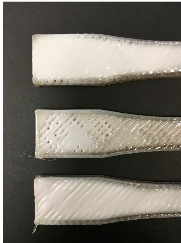
Figure 12. Close up of rPET water bottle tensile bars 3D printed with the same print settings. Inconsistent extrusion caused both under extrusion (top, middle) and over extrusion (bottom), with under extruded sections resulting in macro voids that decreased the UTS of the tensile bar.
