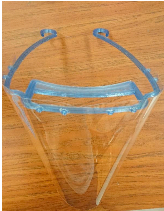
Figure 15. Recycled PET pellets used to 3D print a face shield.
