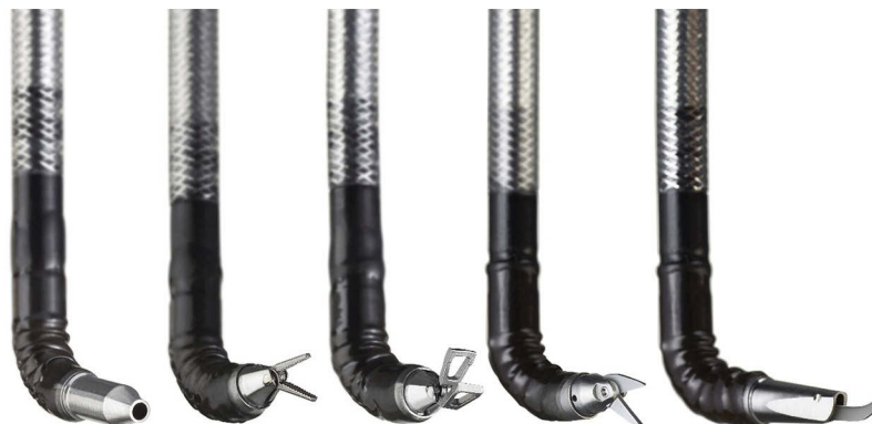
Figure 2 Microlaryngeal Instrumentation available for the Flex robotic system including laser attachment, alligator grasper, triangle forceps, micro-scissors and sickle knife.
