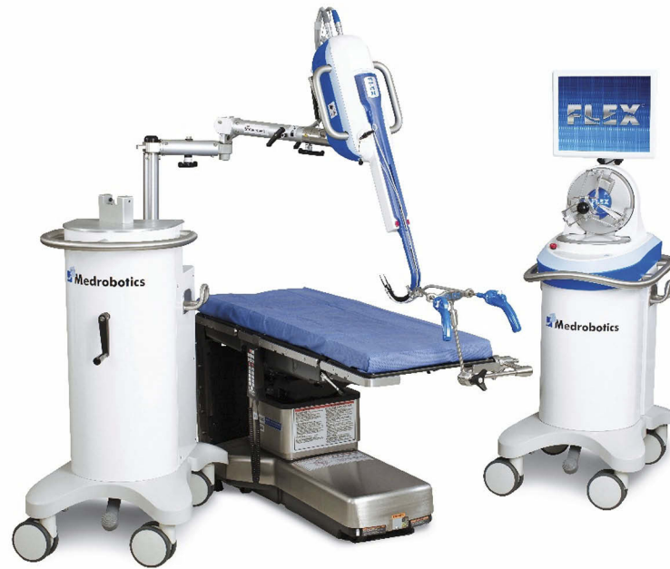
Figure 1 Medrobotics Flex 3D scope with alligator grasper and triangle forceps which demonstrates the ability for the robot to manipulate in a non-linear fashion.
