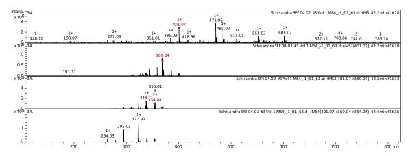
**Figure 3.** Collision-induced dissociation (CID) spectrum of the schisandrin B (gomisin N, isokadsuranin) from *S. chinensis*, *m*/*z* 401.07.
