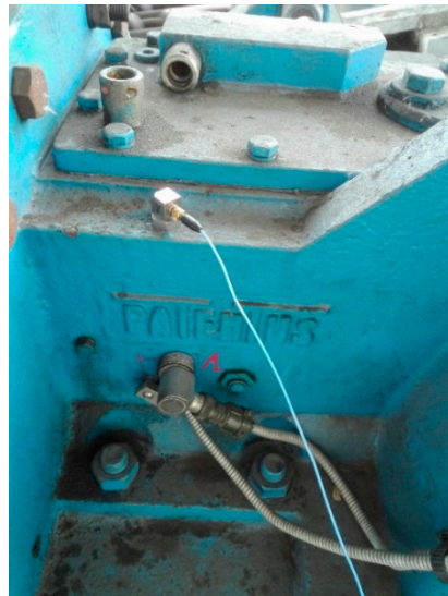
Figure 10. Measurement point 1—housing of 1st-stage transmission—bevel gear.
