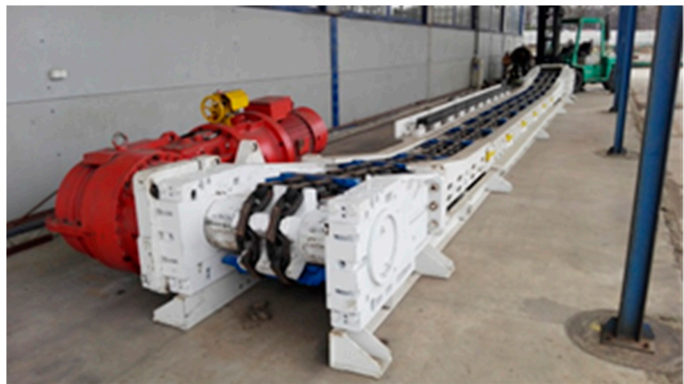
Figure 2. The test transmission installed in the scraper conveyor.
