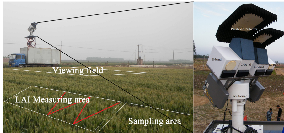
Fig 13. The observation scene (left) of the TMMR instrument (right).
