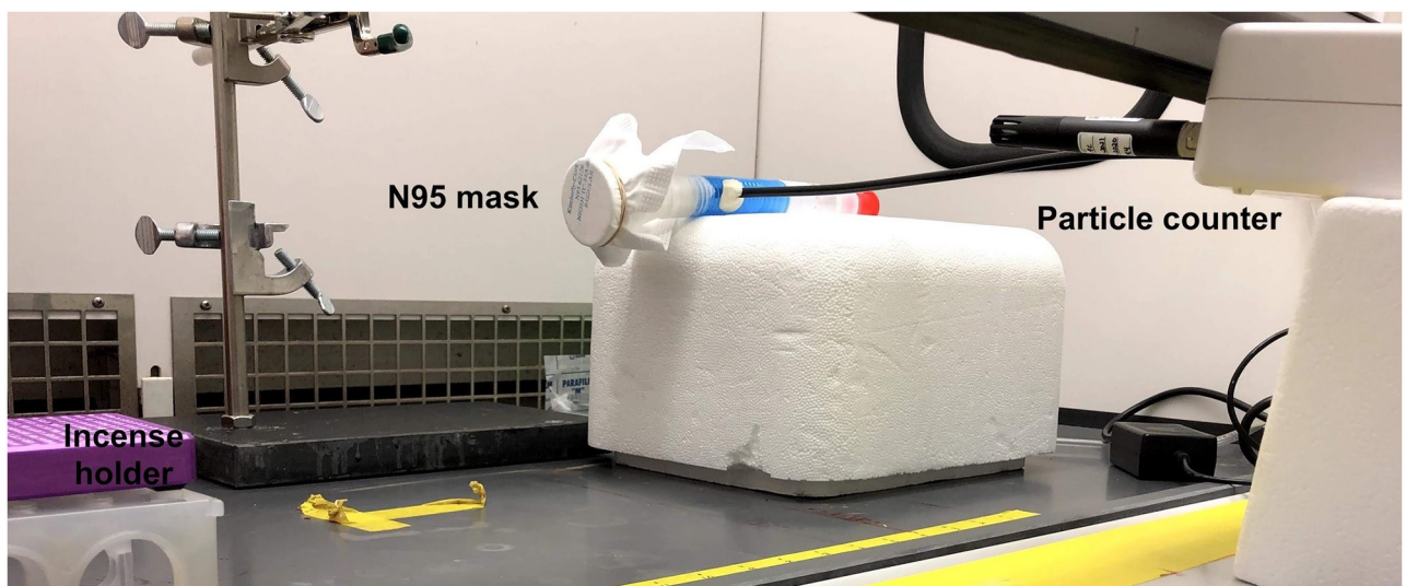
Fig 3. Filtering efficiency test setup to test filter efficiency of a N95 mask using LightHouse handheld particle counter to detect particles of size 0.3\ \mu\text{m} — 10\ \mu\text{m} produced by burning an incense stick.
