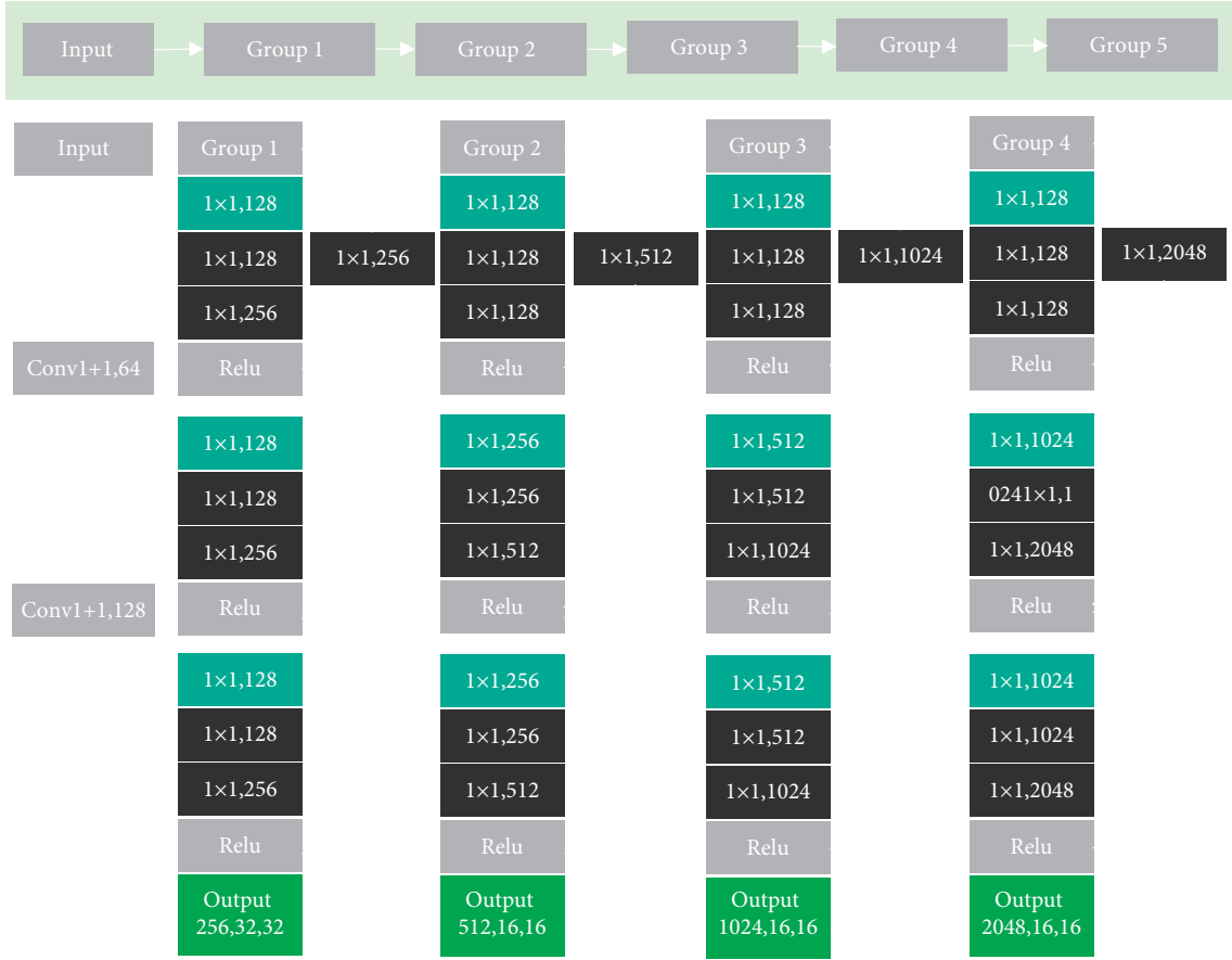
FIGURE 3: The structure diagram of optimized ResNet network.
