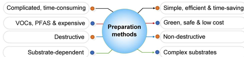
Fig. 4. Challenges of preparation methods for commercialization and widespread practical applications of SH surfaces.
