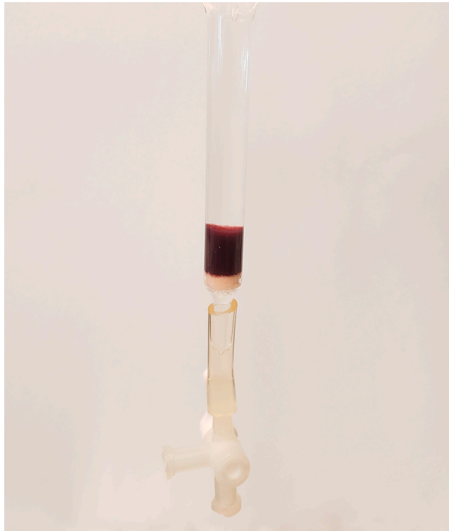
Figure 2. The Ni 2+ -NTA agarose resin appears dark purple in colour after the binding of RCs
