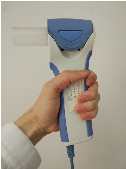
Figure 1 The handheld “disposable pneumotachograph” spirometer.
