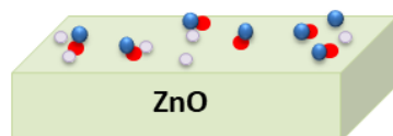
Figure 8. The possible mechanism of CO adsorption on Al-doped ZnO nanorod-coated microcantilever surface. Here, Al atoms (red circles in Figure 8) replaced Zn atoms on the topmost layer of the slab due to the fact that bonding between Zn and O in ZnO crystal lattices is weaker than that those between Zn–Al [13]. (a) CO exposure causes the desorption of undissociated H 2 O molecules, and (b) simultaneously, CO molecules are absorbed on the Al-doped ZnO nanorod surface.
