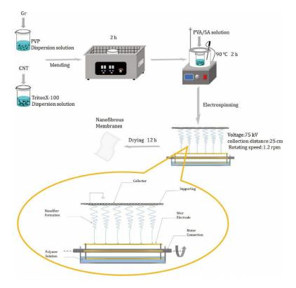
Figure 1. Process of the preparation of linear electrospinning nanofiber membranes.
