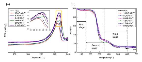
**Figure 8.** Characterization of thermal properties of PVA/SA/Gr/CNT nanofiber membranes: (**a**) DSC of nanofibrous membranes as related to Gr-CNT ratios, and (**b**) TG of nanofibrous membranes as related to Gr-CN ratios.
