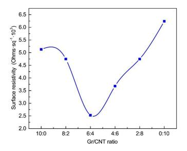
**Figure 5.** Surface electric resistivity of PVA/SA/Gr/CNT nanofibrous membranes as related to the Gr-CNT ratios. (Control: The surface resistivity of the PVA/SA nanofiber membrane was  $7.58 \times 10^9 \ \Omega/m^2$ ).
