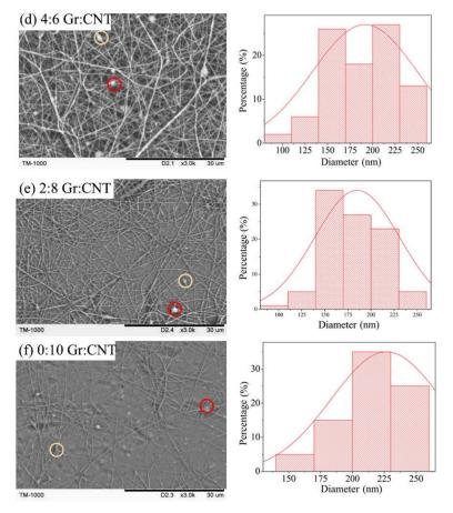
**Figure 3.** SEM images and diameter of PVA/SA/Gr/CNT nanofibers membranes with the Gr-CNT ratios of (a) 10:0, (b) 8:2, (c) 6:4, (d) 4:6, (e) 2:8, (f) 0:10.
