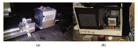
**Figure 1.** (a) Photograph of the source holder and the Neo sCMOS camera in the dark-box. (b) The Neo sCMOS in the LD Didactic X-ray apparatus (554 800)—The blue lines are for the water cooling circuit, which is not necessary for operation in the dark box.
