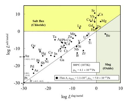
**Figure 2.** Enlarged section near the origin, taken from Figure 1, showing the distribution of elements among slag (oxide), salt flux (chloride), and metal phases under the simulated atmosphere of the aluminum melting process.
