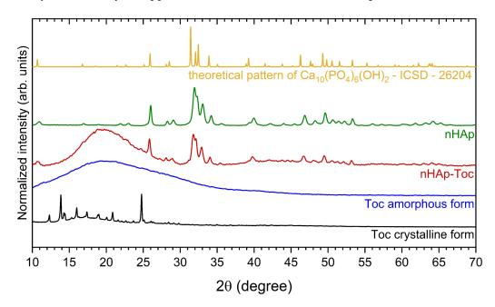
**Figure 1.** X-ray powder diffraction (XRPD) patterns of the crystalline Toceranib (Toc, black line) and amorphous Toceranib (Toc, blue line), the nanohydroxyapatite modified with Toceranib (nHAp-Toc, red line) and the nanohydroxyapatite (nHAp, green line) together with the reference hydroxyapatite pattern (ICSD—26204, yellow line).
