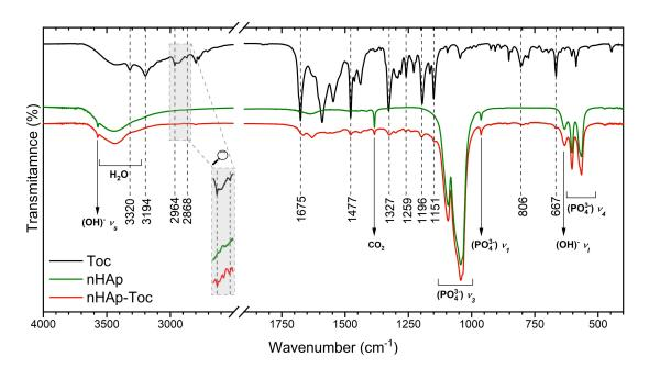
**Figure 2.** Fourier-transform infrared (FT-IR) spectra of the Toceranib (Toc, black line) nanohydroxyapatite (nHAp, green line) and nanohydroxyapatite modified with Toceranib (nHAp-Toc, red line).
