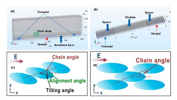
**Figure 2.** (a) Geometry of the 3D model for simulating the tumbling motion of pearl chain in a flow condition. (b) Geometry of the 3D model same as the experimental setup of Singh et al. [14] for simulating the alignment of ellipsoidal particles. (c) Illustration of ellipsoidal particle alignment in chain configuration. (d) Illustration of ellipsoidal particle alignment in stacked configuration.
