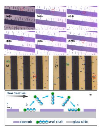
**Figure 1.** Optical images showing the tumbling motion of particle chains. A chain of four particles circled in red moves with the flow in a gap region ( $\mathbf{a}$ ) near the edge of an electrode ( $\mathbf{b}$ ), above the electrode off to the upper side ( $\mathbf{c}$ ), at the center the electrode ( $\mathbf{d}$ ), off the lower side ( $\mathbf{e}$ ), and near the other edge of the electrode ( $\mathbf{f}$ ).
