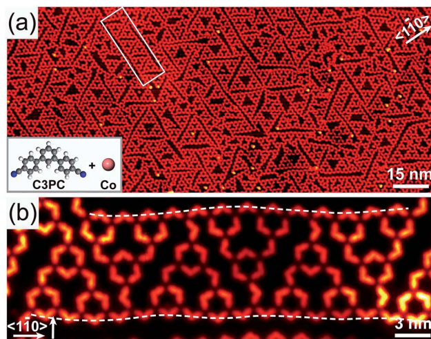
Fig. 4 C3PC-Co-STs formed at high molecular coverage. (a) Overview of irregular network formed by C3PC and Co coordination. The molecular model of C3PC is shown in the left inset. (b) Detailed STM image showing a strip of curved C3PC-Co-ST-2 array indicated by the white rectangle in (a). Both sides of the slightly distorted array are highlighted by dashed curves. Scanning parameters: (a) constant-current mode, V_B = 1.8 V, I_t = 17.5 pA; (b) constant-height mode, V_B = 10 mV, I_t = 15.4 pA.
