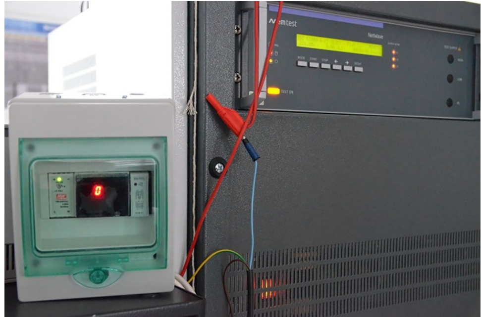
Fig 13. ELSA device during EMC tests.
