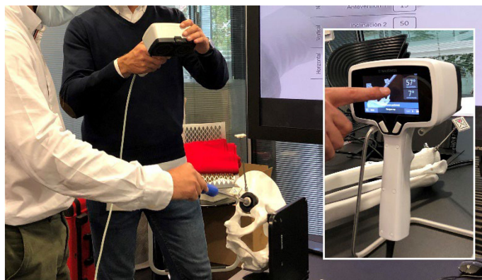
Figure 2. One of the volunteers performing the test. In the square, the navigator providing information on inclination and anteversion.
