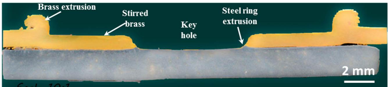
**Figure 6.** Macro image of an FSSW steel/brass joint showing the different zones using a total of 167 revolutions (rpm = 1000 and dwell time = 10 s).
