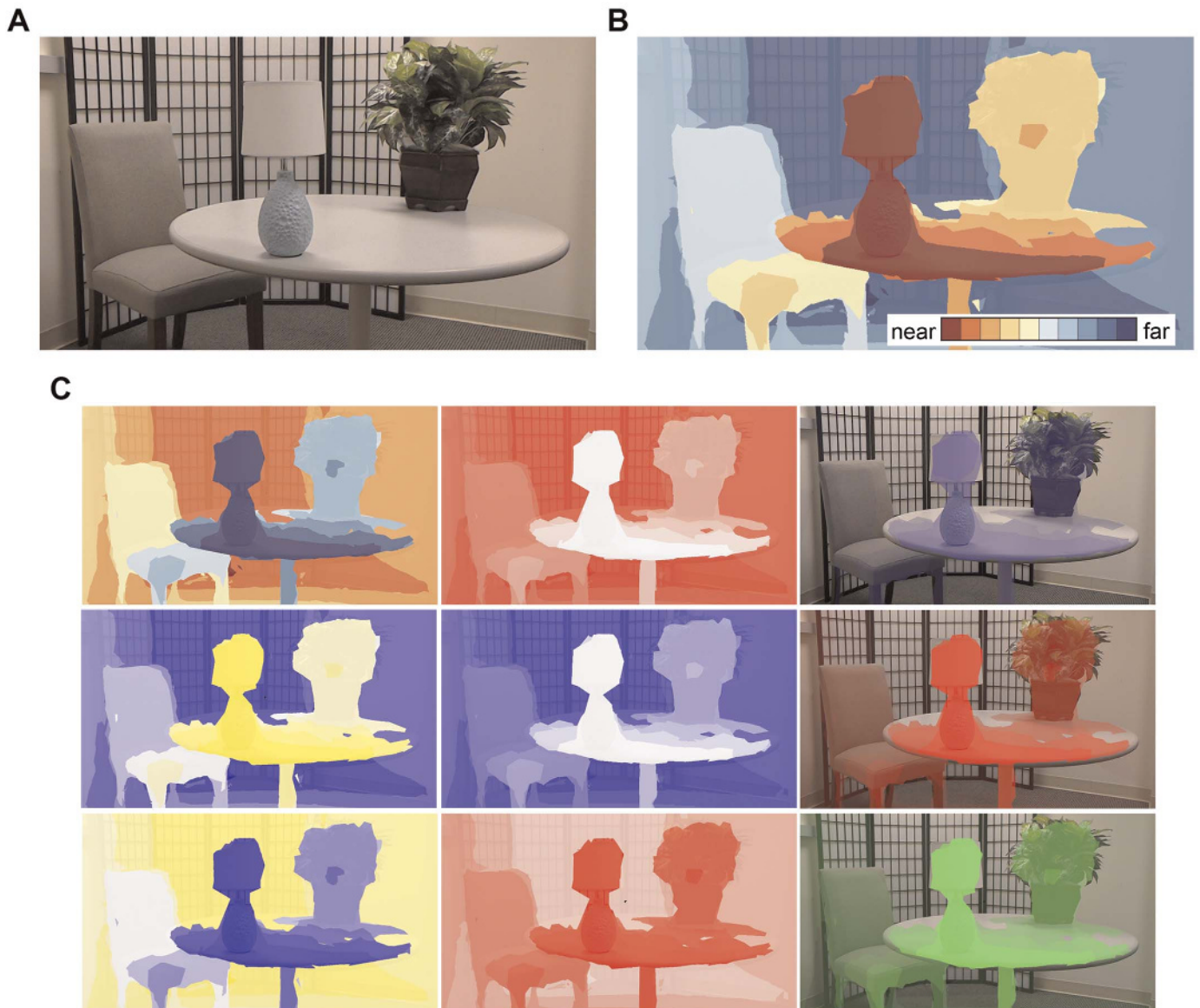
FIGURE 2. Augmented reality application. (A, B) The HoloLens creates a 3D map of the physical environment (A) and can overlay an augmented stereoscopic view (B). The example overlay shows nearby surfaces ( <2.0 m) as warm colors, and farther surfaces (2.0 m and farther). This is the red-to-blue augmented reality (AR) used in Experiment 2. (C) Several other example views of the same scene demonstrate how the color and intensity can be customized for individual users. These is a subset of the options presented to participants in Experiment 1. All examples were captured from the HoloLens using the scene camera positioned between the user's eyes.
