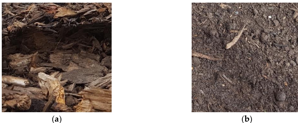
Figure 3. Applied filling materials, (a) A mix of stumpwood chips and pine bark (CB), (b) a mix of stumpwood chips, pine bark, and green waste compost (CBC).
