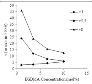
Figure 3 Media penetration velocity at pH 1-8 in polymers comprised of 1-10 mol% EGDMA.
