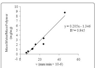
Figure 4 Equilibrium media content at pH higher than pK<sub>a</sub> of AA as a function of media penetration velocity in the polymers comprised of 1-10 mol% EGDMA.
