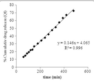
Figure 9 Zero order release kinetics of optimized formulaion having 3.5 mol% EGDMA at pH 8, having drug concentration of 3.2 mg/mL.
