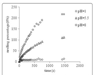
Figure 1 Media sorption profile for optimized concentration of the cross linker (3.5 mol%) exhibiting effect of pH.
